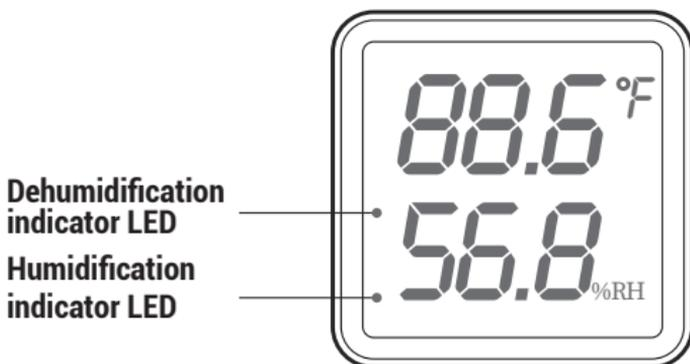
**Humidification indicator LED:** If humidity Control Function selected humidification mode, the indicator LED is on, otherwise off.
