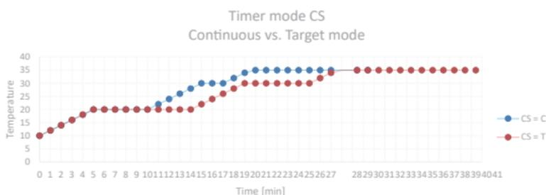
From the graph, we can see that when TR=1, the continuous timer mode (the blue line), the stage control time H01~H03 is continuous time, 0...10, 11...17, 18...29, total is 29 minutes; When TR=2, the target timer mode (the red line), the stage control time H01~H03 is only started when the current temperature reaches the setting temperature of the current stage, such as 5...14, 19...25, 32...35, and total is 39 minutes.
